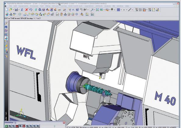
TopSolid'Cam enables the complete programming of parts in turning, milling and 5 axes operations.
